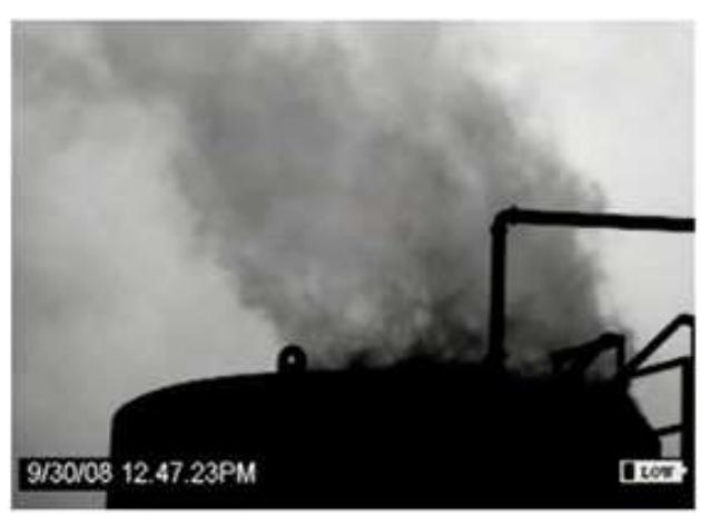
**Methane is not visible to naked eye, but can be “seen” with infra-red cameras.**
